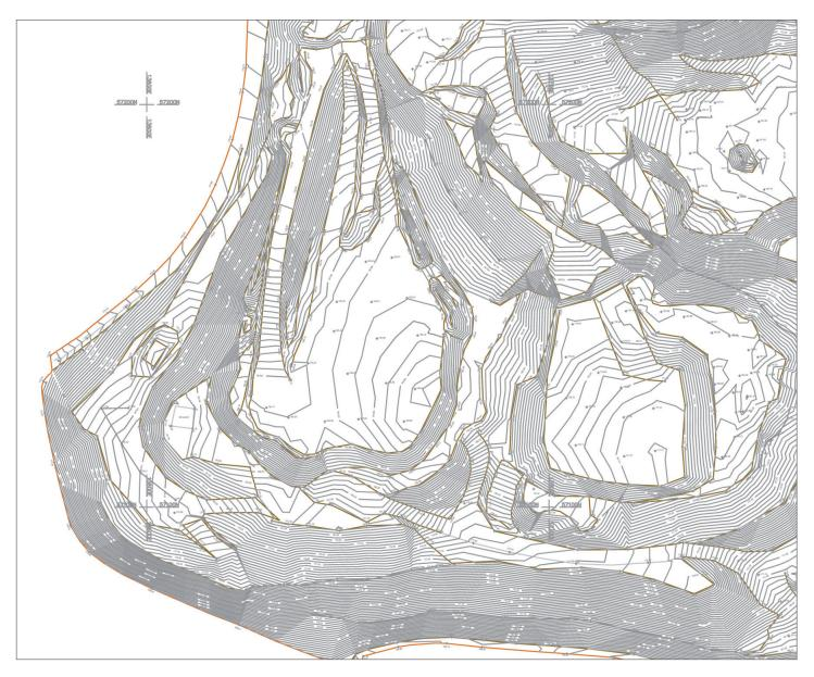
An extract of part of digital terrain model (DTM) of a regeneration scheme in the English Midlands. A large earth moving exercise was undertaken by the local authority who asked the survey company to provide continual volumetric calculations of smaller areas to check the quantities the earth moving contractor was submitting. Periodically full surveys were required to check against the design model and check compaction against the original ground model.
